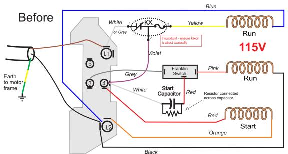
Note: The terminal positions may vary from that shown on AMF diagrams. White wire from L1 to Klixon may be Grey. These drawing are based on an actual motor from an 82-90XL American mains cables will be Black=Active, White=Neutral.
